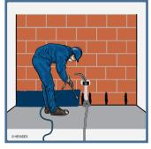
**Floor/wall connections** are a vital area to seal in order to meet high levels of airtightness, once a floor covering is in place it's very difficult to rectify leaking connections. Apply Blowerproof to dust free, solid surfaces fill cracks or gaps beforehand: large holes and joints > 5mm can be repaired with a fast setting cement based product or PU foam, small holes and joints 2-5mm can be sealed with Blowerproof Liquid Brush.
