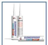
**Blowerproof Brush Blue—cartridge** the 300gram cartridge allow precise and targeted application of Blowerproof Brush Blue to areas such as window jambs, door jambs penetrations and difficult to reach applications. Apply as a single or double bead then brush finish to ensure a complete seal. The product can be used for sealing between boards and for perimeter joints, ensure the total applied depth does not exceed 10mm.
