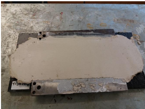
Plate 3.4.3: After application of the bonding compound.
