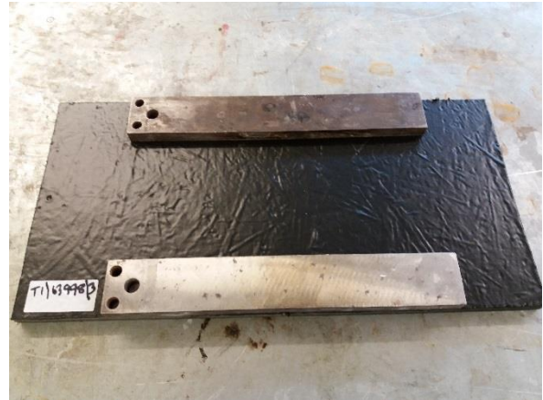
Plate 2.4.2: Lot 3 Showing 16mm thickness spacers.
