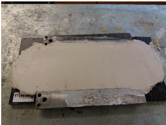
Plate 3.4.3: After application of the bonding compound.
